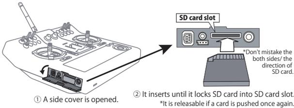
2. After inserting the new SD card into the transmitter, turn on the power switch. You will see the word "FORMAT" if you have not previously used this card in the transmitter.
