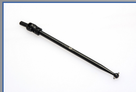
24.CKD0202 Center Rear Universal Joint Shaft
