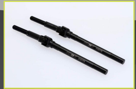
24.CKQ0206 Front Universal Joint 175/210WB For 4WD (2 Stk.)
